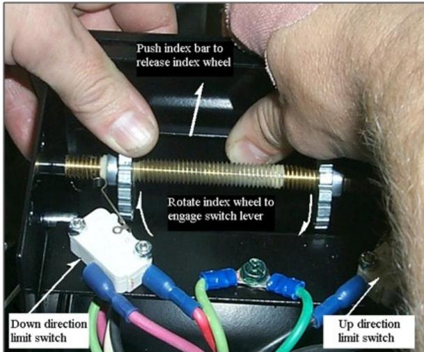
3. Press the black index locking bar away from the down direction index wheel so it can rotate freely. Rotate the wheel until the switch “clicks” indicating that the switch is active
