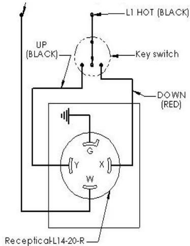
Wiring schematic for LynRus CW3 hoist with optional pigtail
